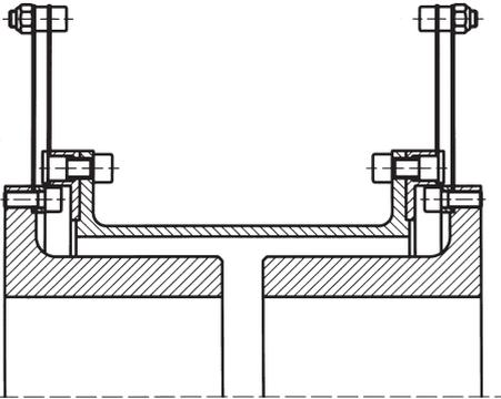
CENTADISC-M – short version with hubs inside the tube. Radial exchange not possible.
