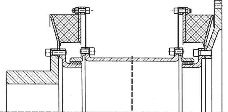
CENTADISC-M-flexible shaft, combined with torsionally soft CENTAX couplings in order to dampen torsional vibrations. Typical area of application: Diesel engines on very soft mounts.
