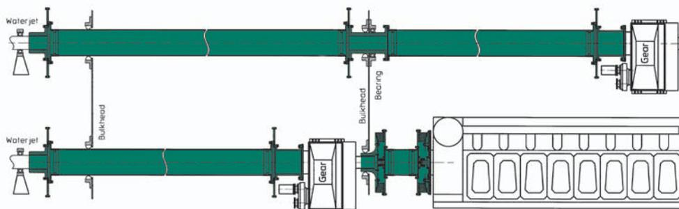
Typical arrangement of CENTA couplings and Carbon Fibre shafts. The first section behind the engines also comprises 2 CENTAX torsional couplings each that tune the torsional vibrations of the system.
